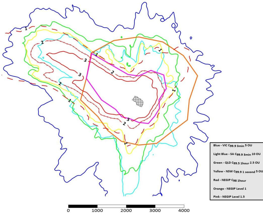
Figure 33. Example of odour modelling results - odour contours and separation distances around the generic piggery site (black hatched area)
