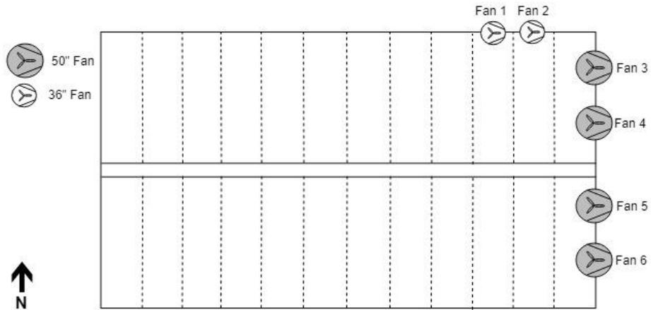
Figure 5. Grower/finisher shed at Farm A – mechanically ventilated with pull-plug effluent system
