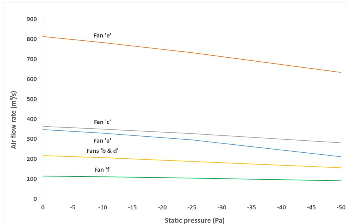
Figure 11. Air flow rate of fans, showing decreasing flow rate as static pressure in the shed becomes more negative
