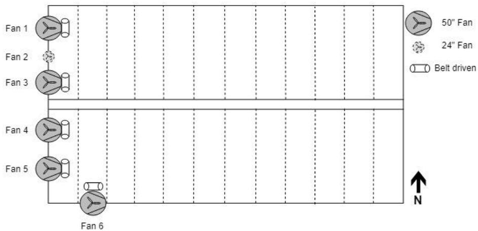
Figure 4. Grower/finisher shed at Farm A – mechanically ventilated with effluent flushing system
