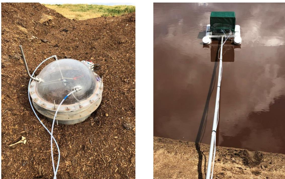
Figure 1. Flux chamber used to capture odour emissions from compost and effluent surfaces
