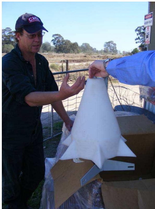
Image 2: Geoff Fisher and Greg Mills (arm) discussing the Sure-Flo® insert. It can be noticed that the insert is not rigid – there is some movement possible side to side on the vertical rod that passes up through the centre of the cone.
