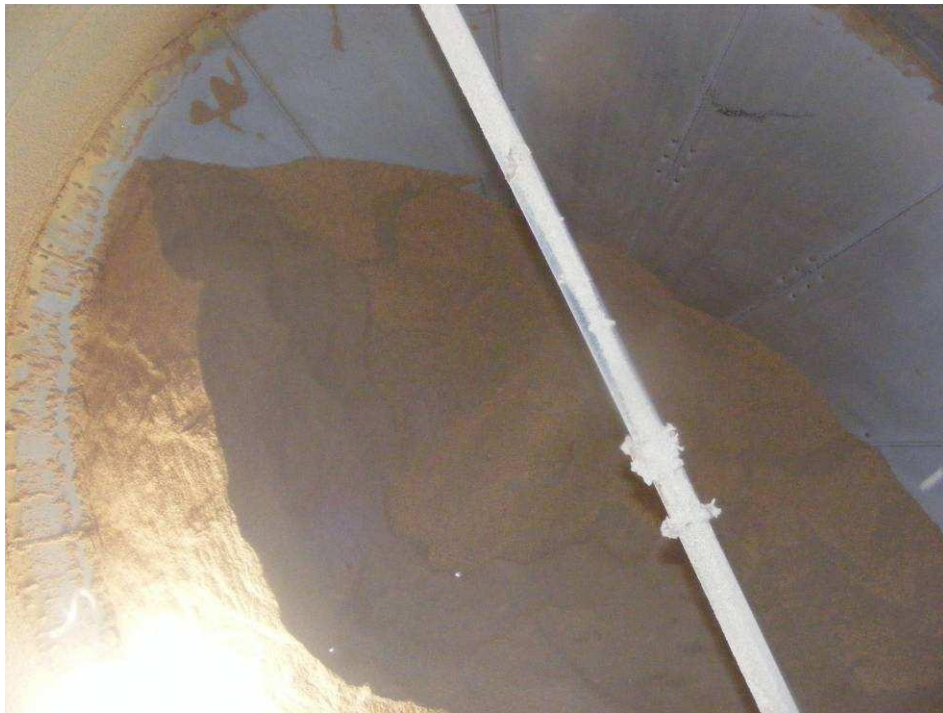
Image 9: The feed in the cone is emptying from one side of the cone, leaving feed piled up on the other side of the cone
