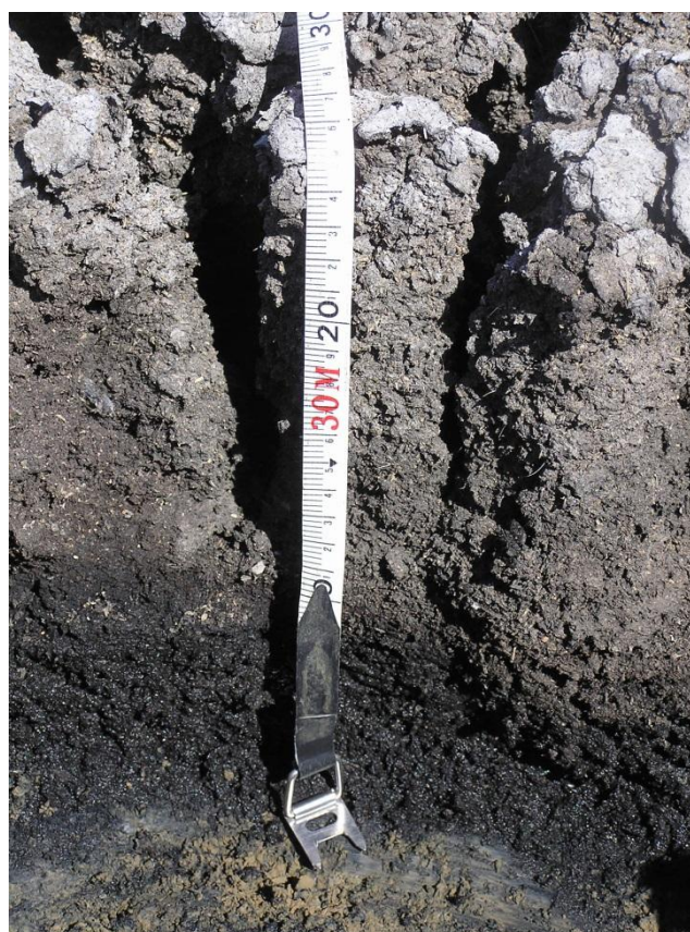
Figure 14: 150 mm of dry manure solids over 100 mm of moist material (test location M2)
