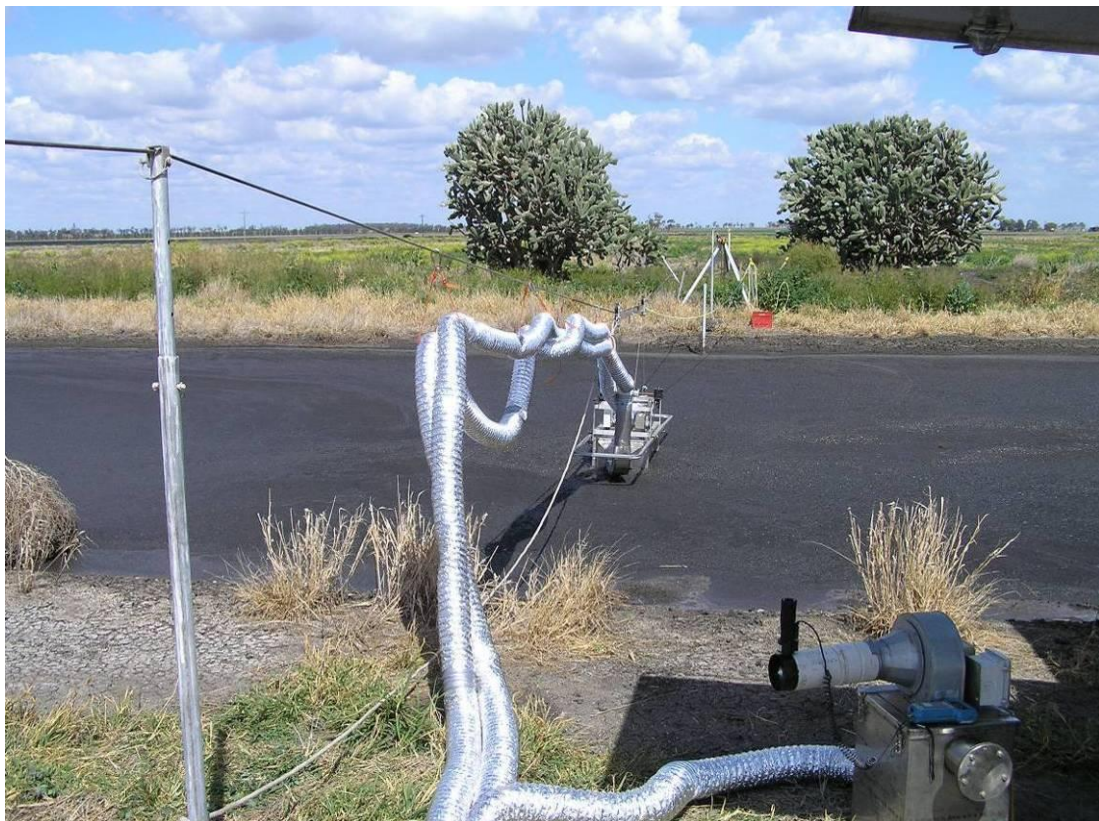
Figure 19: Odour sampling from the upstream end of SEP 3 (active SEP) on 28 August 2012 using the wind tunnel.
