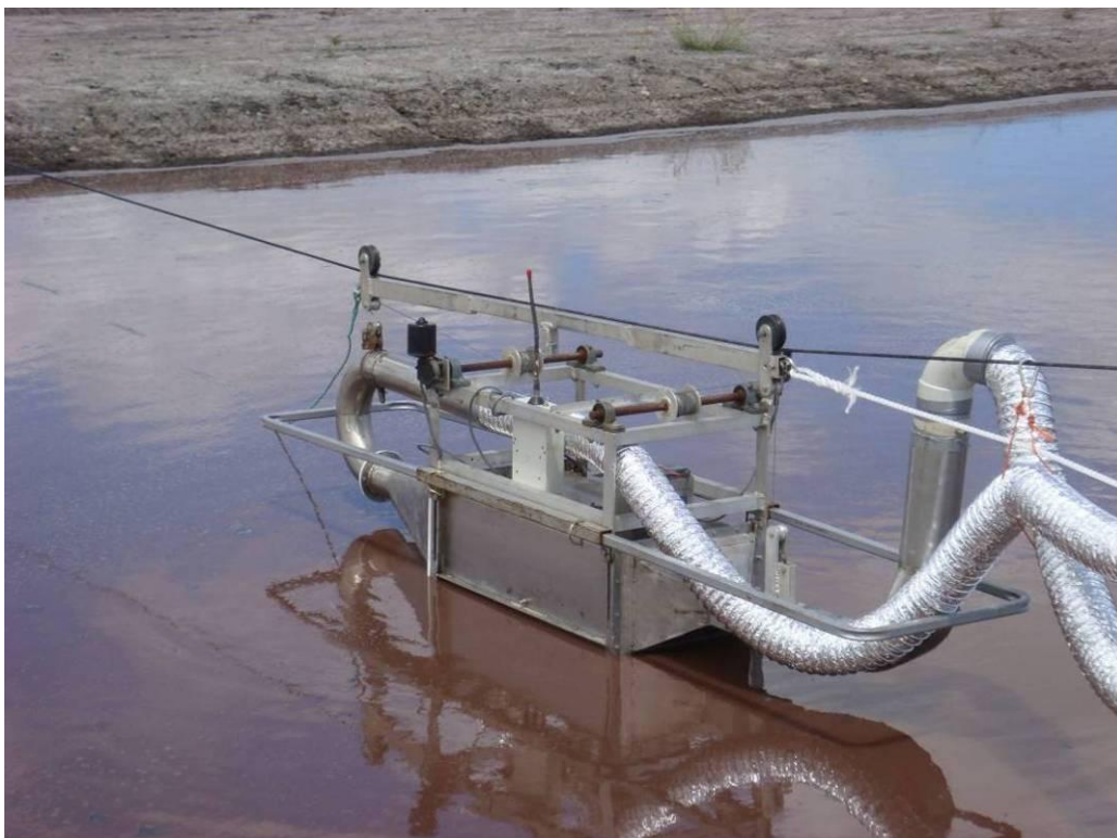
Figure 15: Wind tunnel collecting odour sample from near the eastern end of the SEPS channel (25 November 2010).
