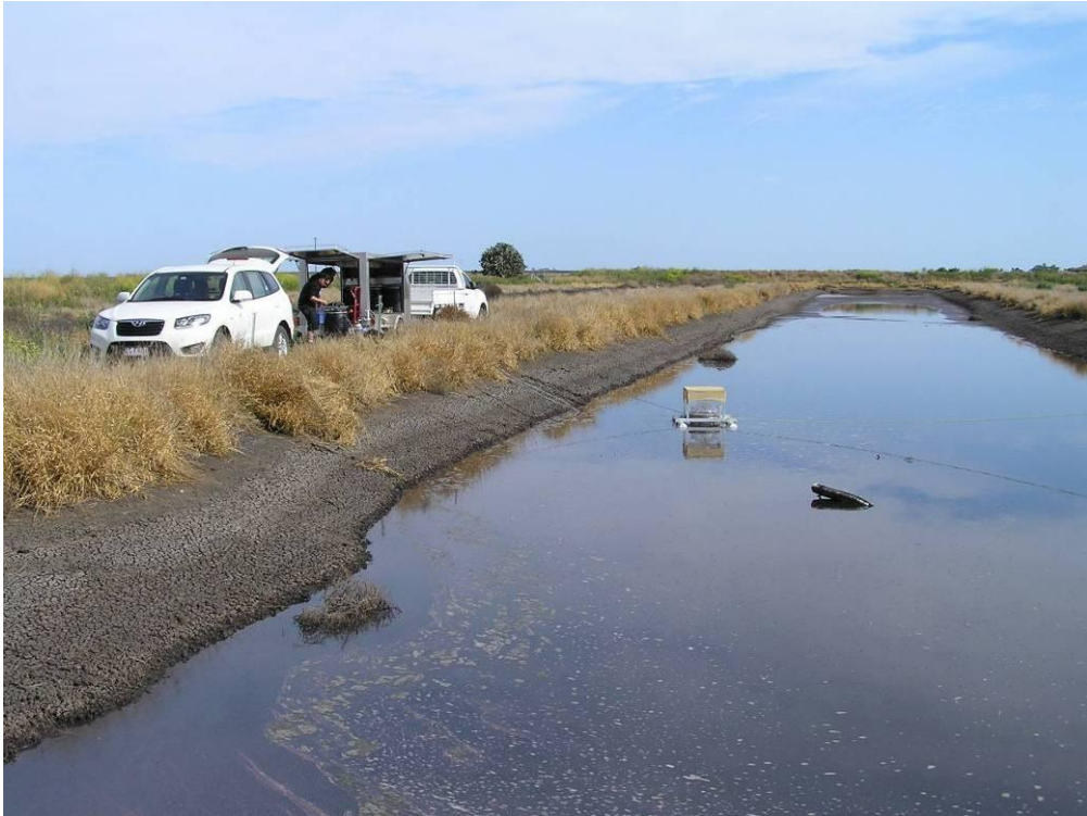
Figure 20: Odour sampling from the downstream end of SEP 2 (drying SEP) on 29 August 2012 using the flux chamber.
