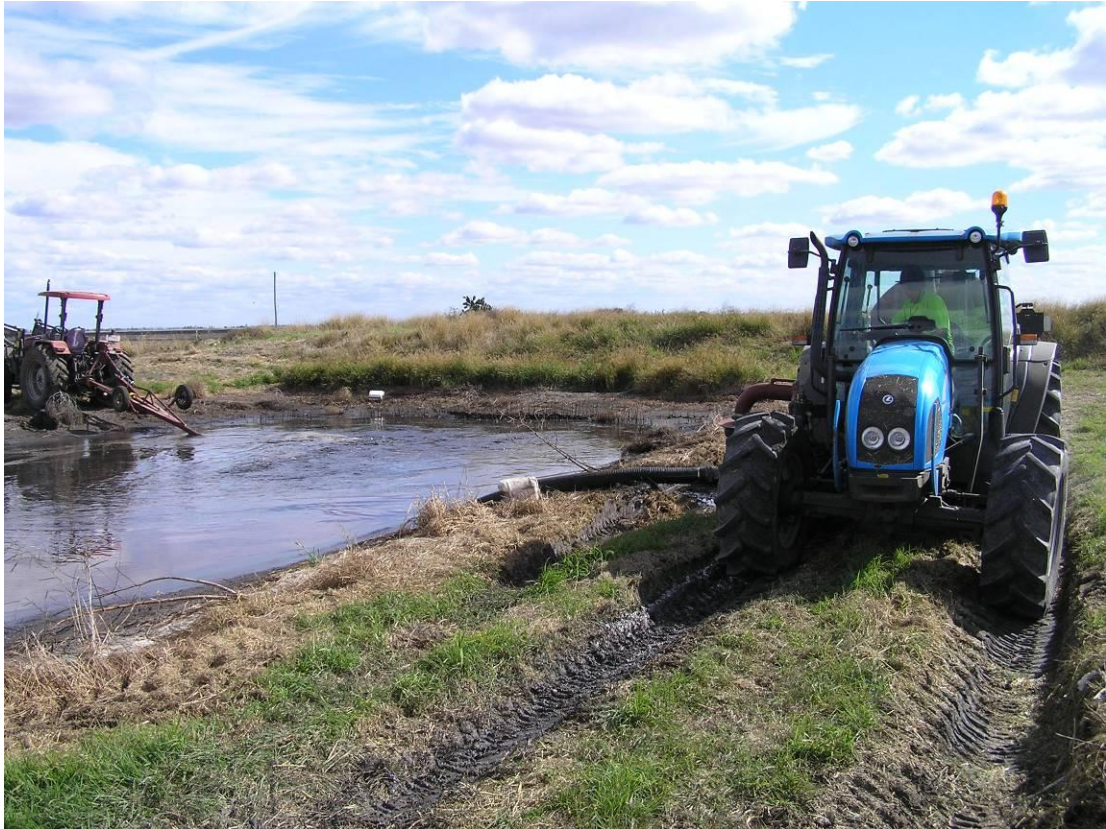
Figure 31: Giltrap slurry spreader and pond stirrer operating near the upstream end of SEP 3.
