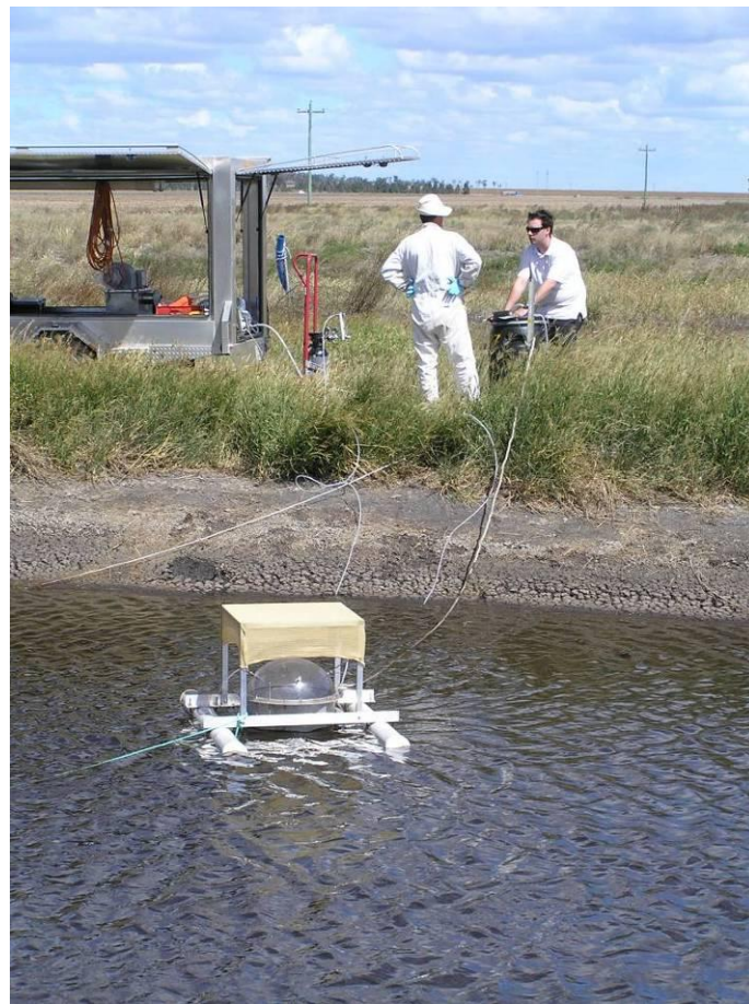
Figure 21: Odour sampling from the return drain using the flux chamber (12 April 2012)
