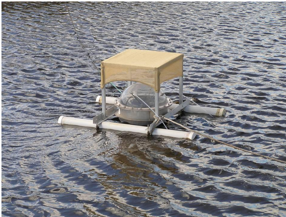
Figure 22: Close-up view of the flux chamber collecting odour sample from the return drain (12 April 2012).
