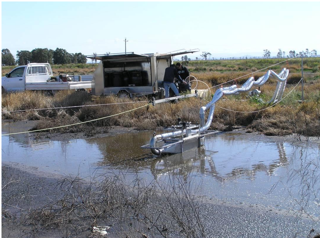
Figure 17: Wind tunnel collecting odour sample from near the western end of the SEPS channel, close to the location where the shed effluent enters the SEPS (28 August 2012).
