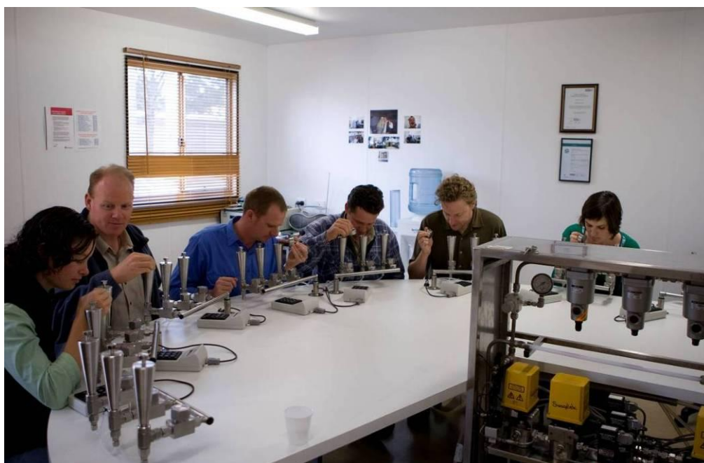
Figure 24: The Agri-Science Queensland olfactometer in operation showing panellists sniffing at ports.
