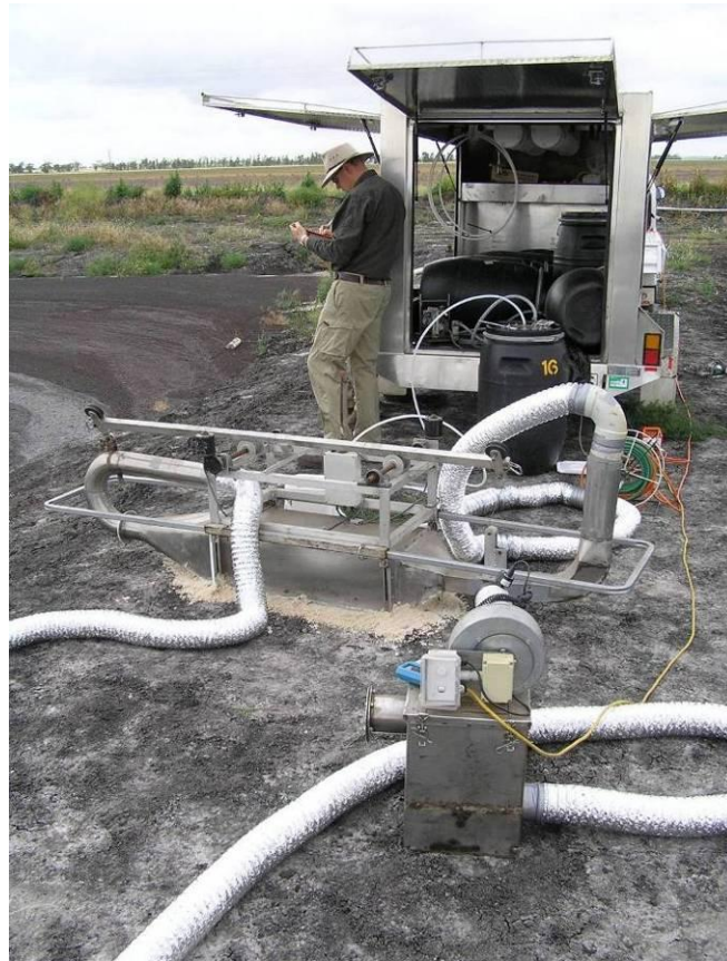
Figure 14: Collecting a blank odour sample using the Agri-Science wind tunnel positioned on a stainless steel sheet adjacent to the SEP channel (November 2011).
