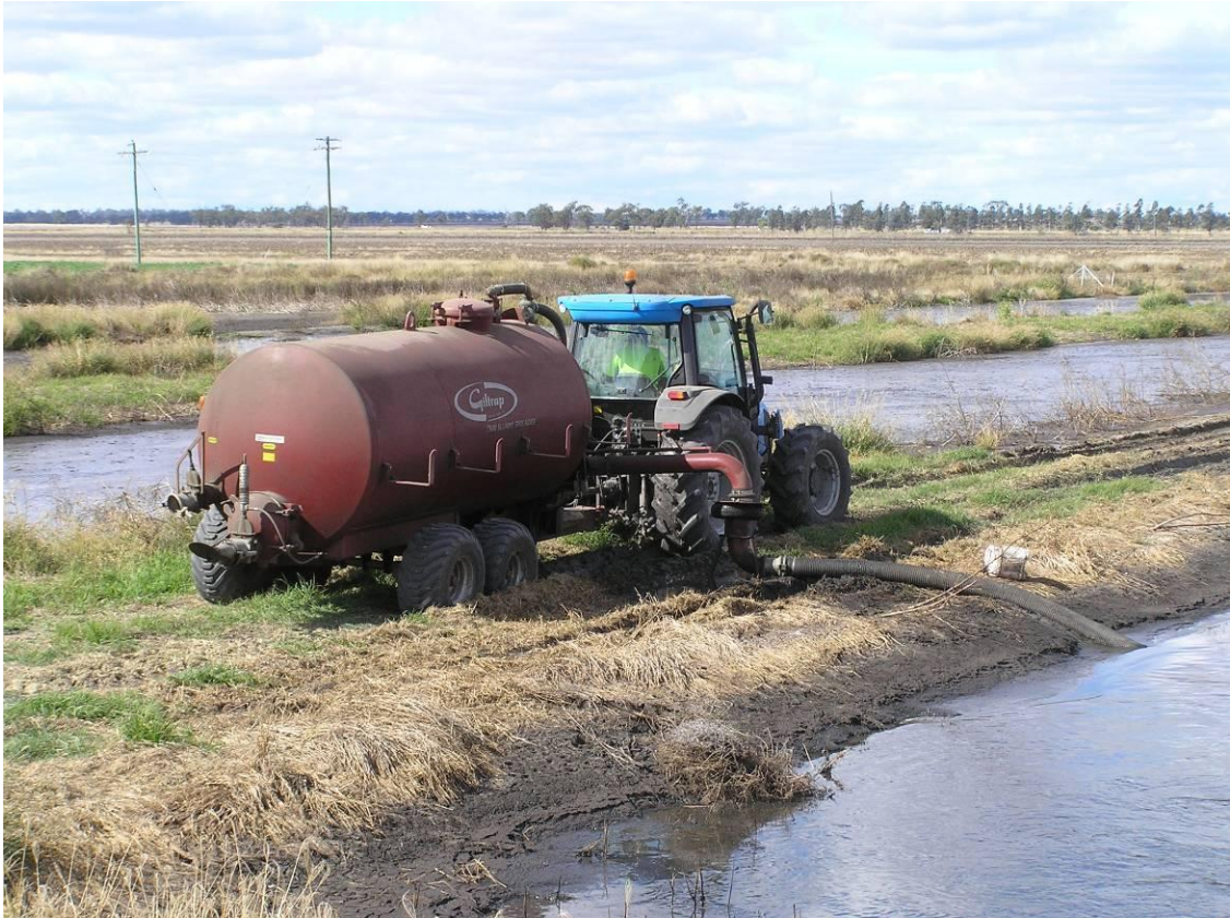
Figure 29: Giltrap slurry spreader lifting agitated slurry from SEP 3.
