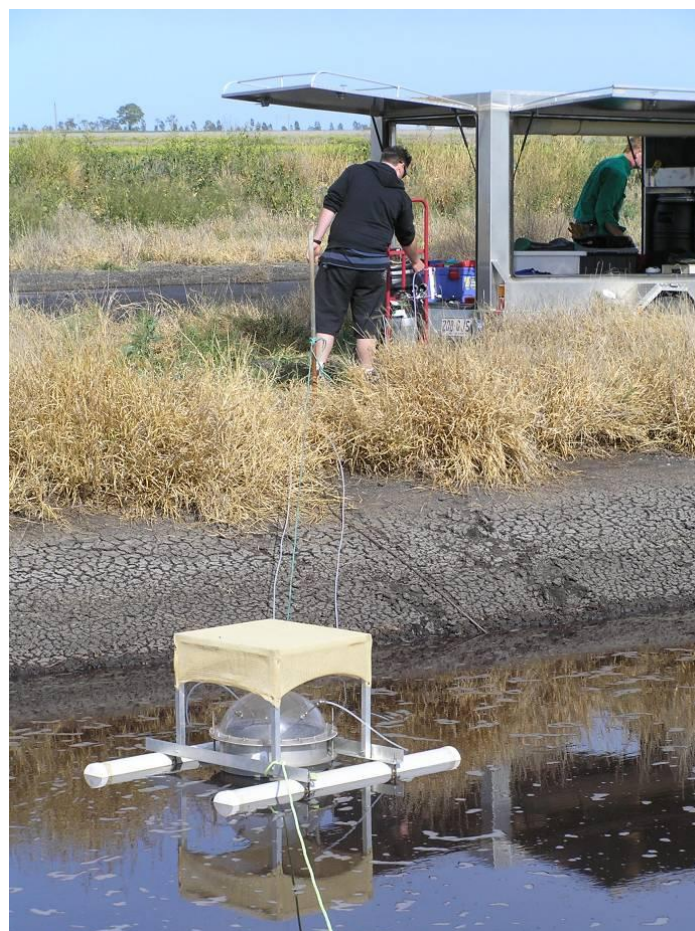
Figure 23: Flux chamber sampling from the drying SEP 2 on 29 August 2012.
